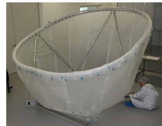
MSTTM MLI fit-check in the STI cleanroom
