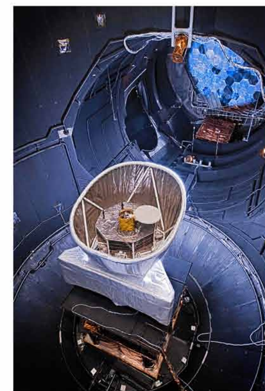
MSTTM with MMO in the large sun simulator at ESTEC
